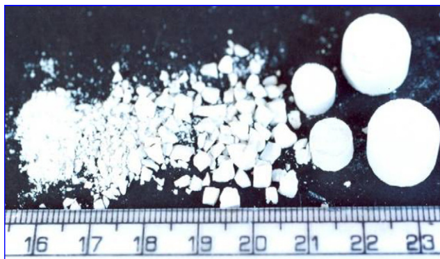
Fig. 1. AP-SiO 2 nanoparticles-based material in the shape of pellets, granules and powder.
